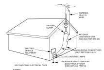
EXAMPLE OF ANTENNA GROUNDING AS PER ANTIONAL ELECTRICAL CODE
